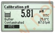
Buffer Contaminated –The offset of the electrode is not in the accepted range. Check if the electrode is broken or clean it following the Cleaning Procedure at the end of this section. Check the quality of the buffer. If necessary, change the buffer.
