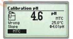
Wrong or Wrong Old Slope – An inconsistency between new and previous (old) calibration is detected.
