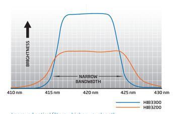
Improved optical filters – higher wavelength accuracy and light throughput
