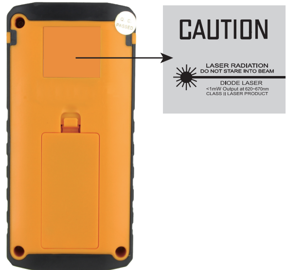
Location of Laser Warning Label
